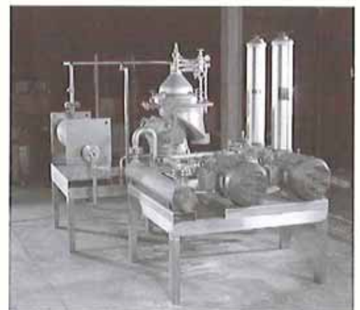
Oil module designed to lubricate, filter and monitor large volumes of oil flow, whilst maintaining the lubricant at a constant temperature.
