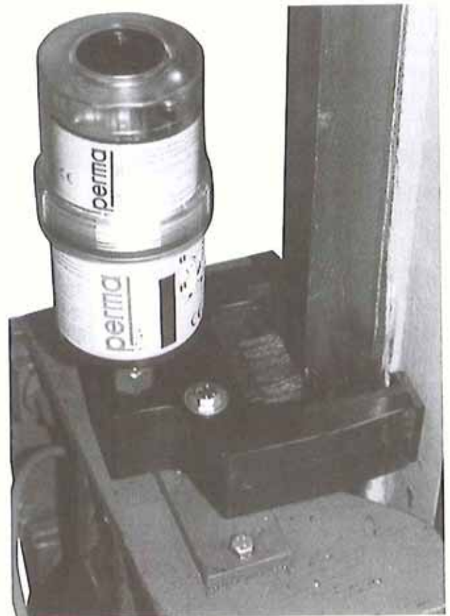
Automatic oil lubrication of sliding guideways with a rail oiler/brush applicator
