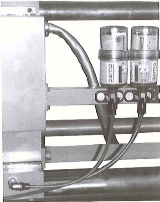
Automatic grease lubrication of slideways and bearings where the lubricators are remotely mounted.
