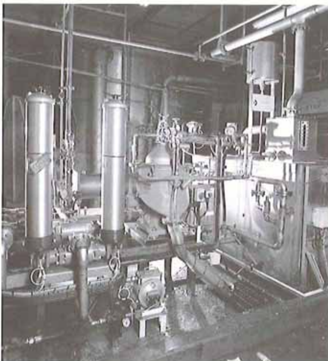
Oil module designed to lubricate, filter and monitor large volumes of oil flow, whilst maintaining the lubricant at a constant temperature.
